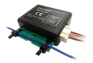
SIMPLE-CAN works in the **listening mode only**, so not all the data available on the CAN-BUS may be received using this solution. **The device automatically sets CAN L/H polarity**, but the calibration has to be always executed during installation process. Connection of previously calibrated unit to another car needs new calibration because the reader **automatically adjusts signal level and speed** to different CAN-BUSes. The device also **automatically adapts to** the found **noise level**.
